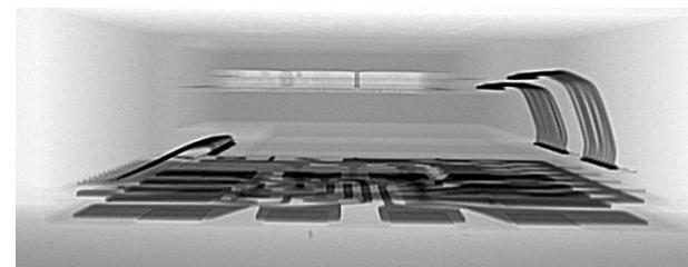
Figure 1.2.2 Package X-ray Side View
