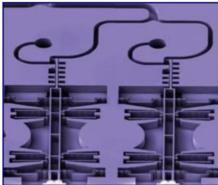
World's fastest MEMS (actuator for cell sorting)
