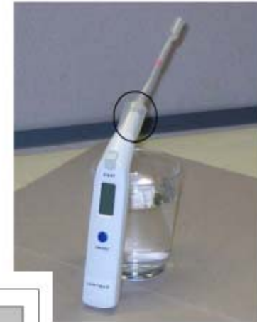
Disposable sensor and reader for home or lab use
