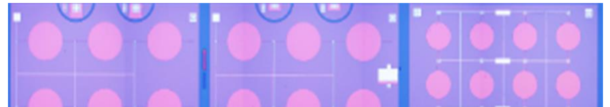
PMUT fabricated on C-SOI substrates
